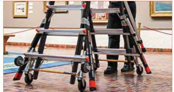
Move the Cage while set up with the Wheel Lift™ casters
